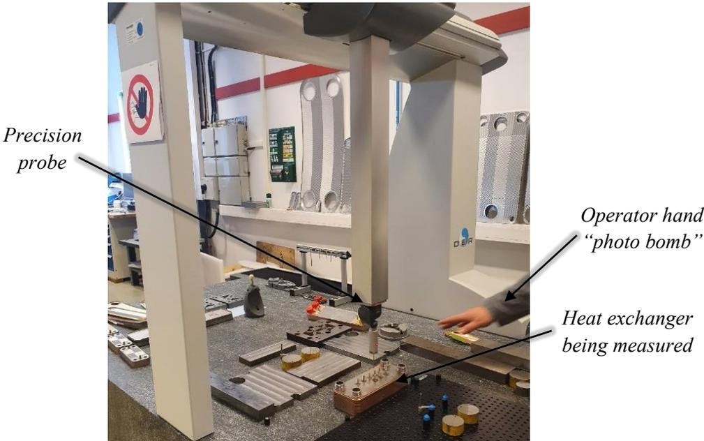
Figure 41: The machine used in the lab to measure the bolt position accuracy.
