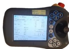
Figure 18: The FlexPendant operator unit. [18]
