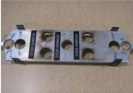
Figure 5: The steel template used to position bolts.
