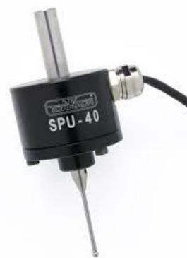
Figure 14: The touch probe. Image from [5].
