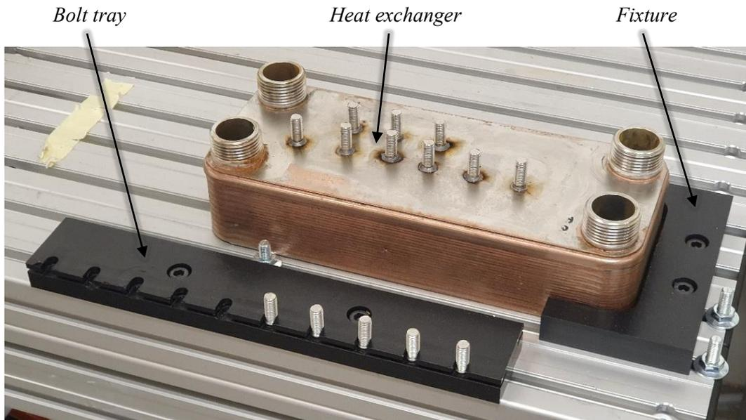
Figure 12: Workstation setup with bolt tray and fixture.
