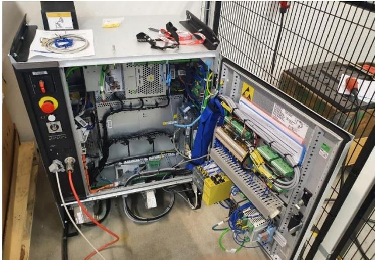
Figure 16: The IRC5 robot controller cabinet.
