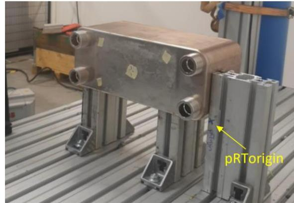
Figure 77: Fixture concept design A – garage test rig.
