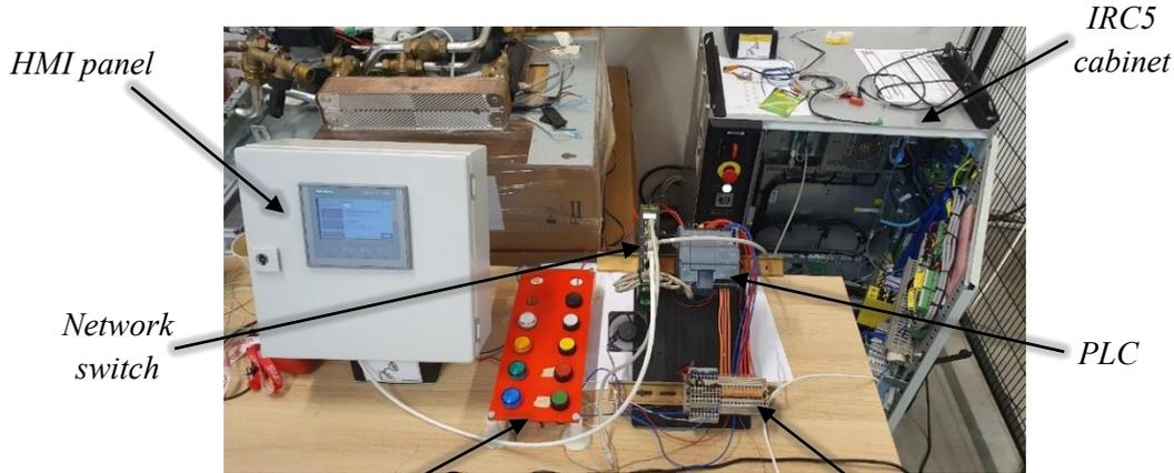
Figure 43: The physical devices setup.
