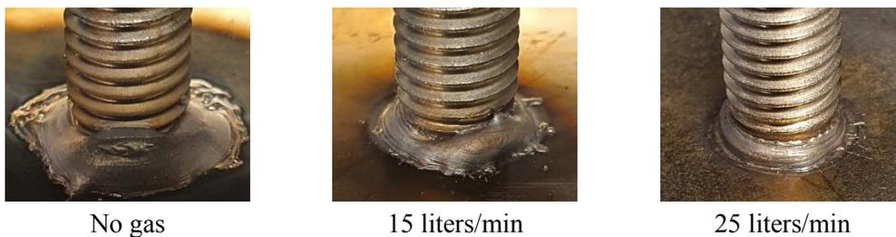
*Figure 36: The weld quality tests, varying the gas flow.*
