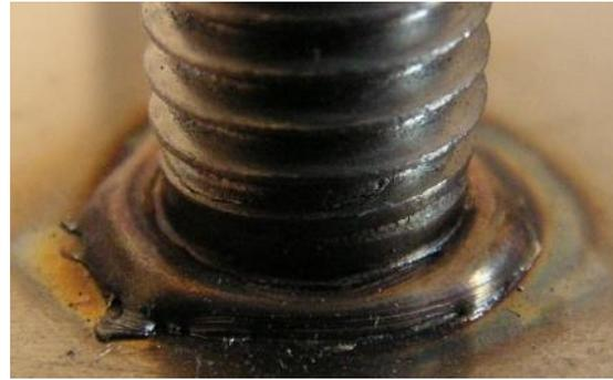
Figure 8: Example of a successful bolt weld.
