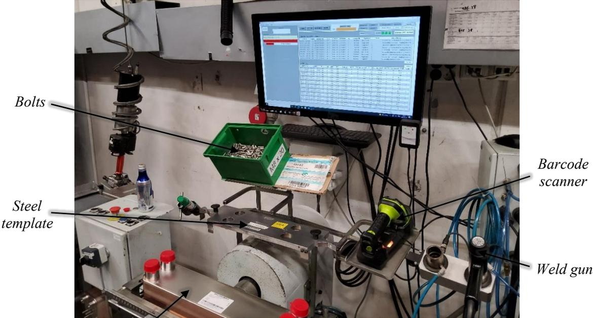
Figure 4: The manual bolt welding work station.
